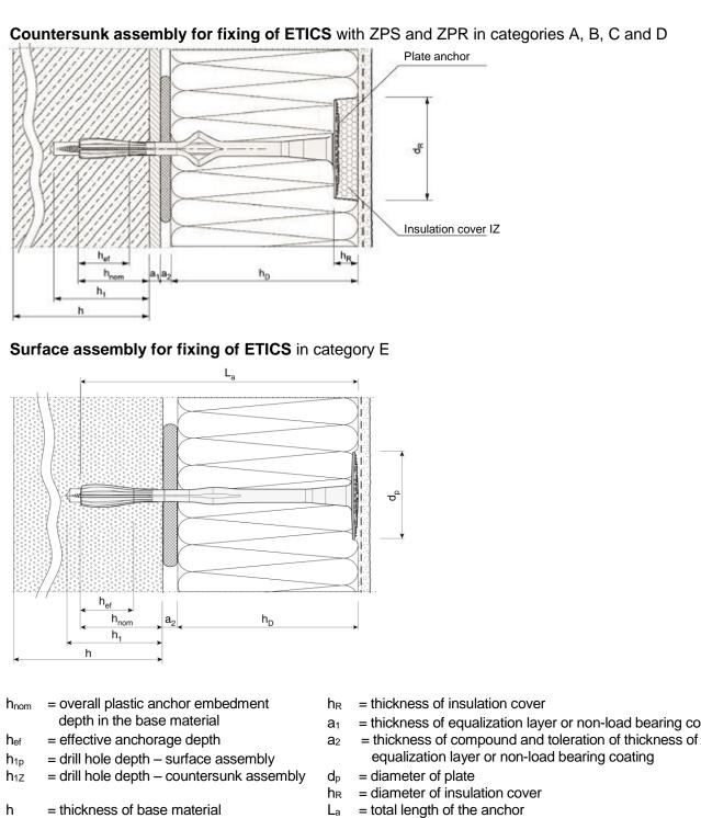
= thickness of insulation material  $h_D$
